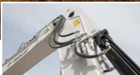
Standard two directional auxiliary hydraulics (1st & 2nd) mounted to the dipperstick, allowing easy connection.
